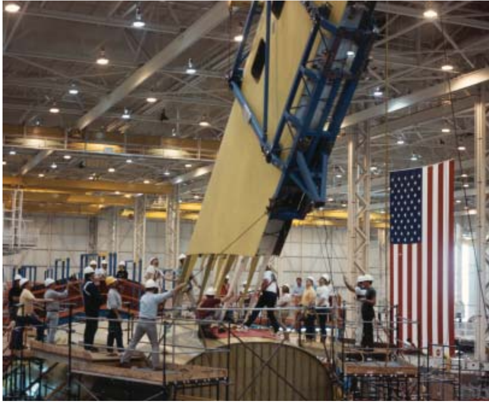
Vertical spars guided to aft fuselage, April 1990. (Boeing)
