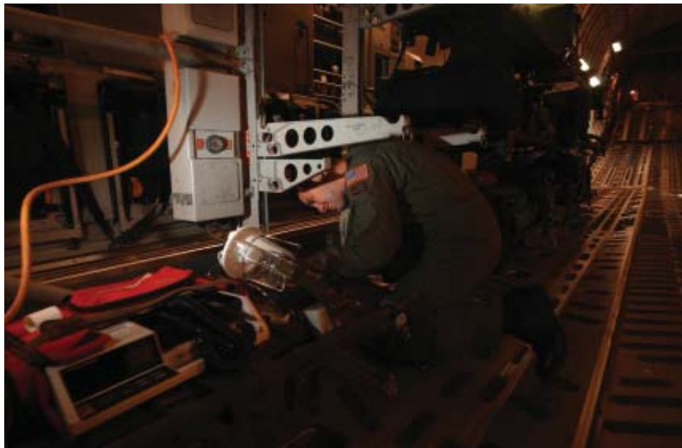
Securing stanchions on a C-17 for litter patients, Ramstein Air Base, Germany, October 2003. (USAF, TSgt Justin D. Pyle)
