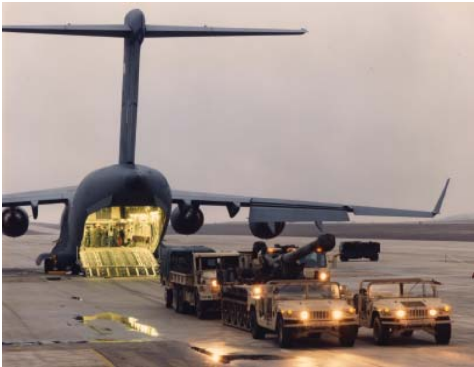
Loading the C-17 with two HUMVEES, a M1102A self-propelled howitzer (62,500 pounds), a 2.5-ton truck with trailer, and a 10-ton Oshkosh truck, Fort Hood, Texas, February 1993. (Boeing)
