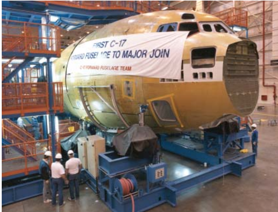
Forward fuselage to major join, February 1990. (Boeing)
