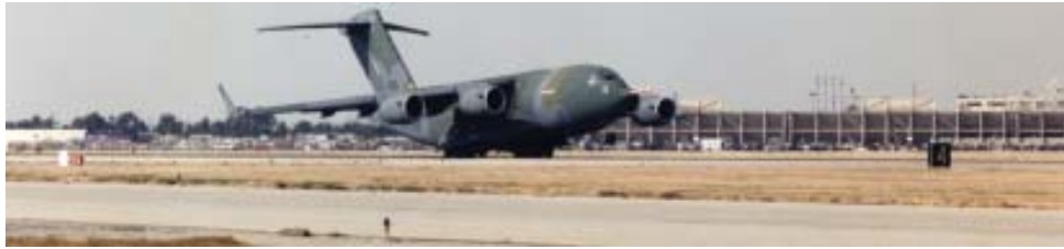
T-1 high speed taxi with nose rotation, 12 September 1991. (Boeing)
