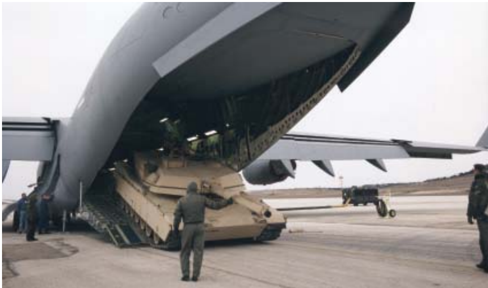
Loading the 130,000-pound M1A1 Abrams main battle tank, Fort Hood, Texas. (Boeing)
