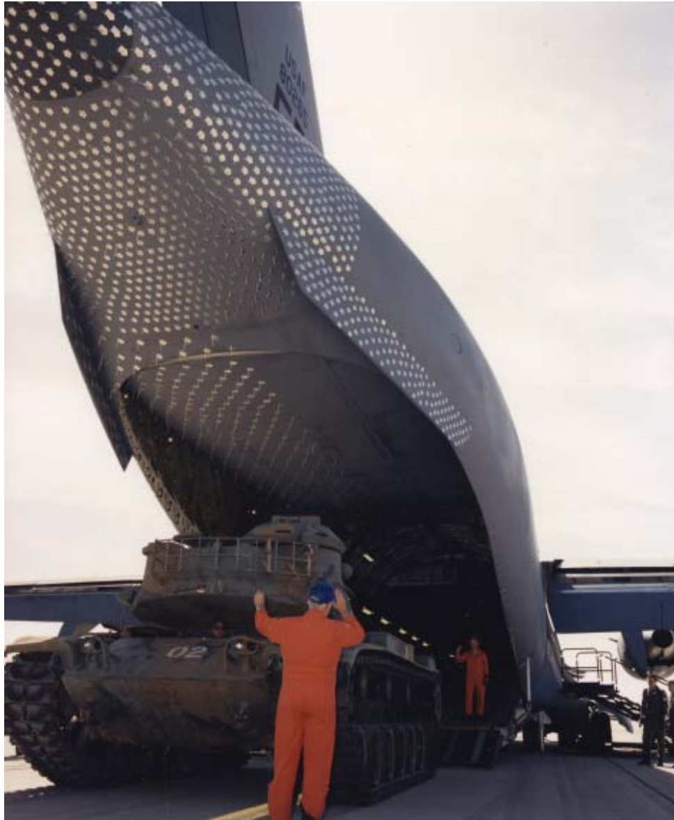
93,000-pound M-60 tank boards P-1. "Tufis" on rear fuselage record airflow patterns, Fall 1993.
