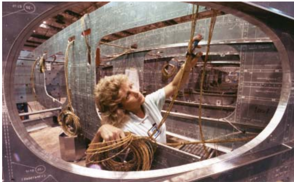
LTV worker installing wire routing. (Boeing)
