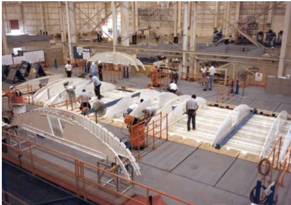
Attaching underfloor bulkheads. (Boeing)
